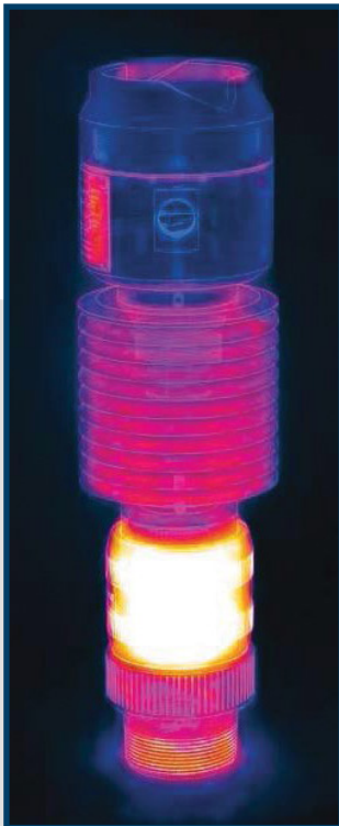
High Temperature Switch (Thermal Image)
